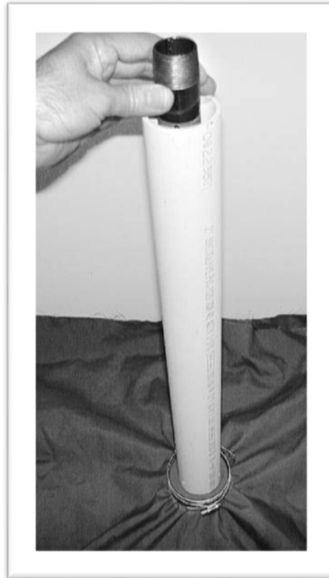
Figure 7 -Drop Tester just before making a test drop. Note that the guide tube is centered on the clamped fabric, and the drop probe is being used as a plumb bob to make the guide tube vertical.
